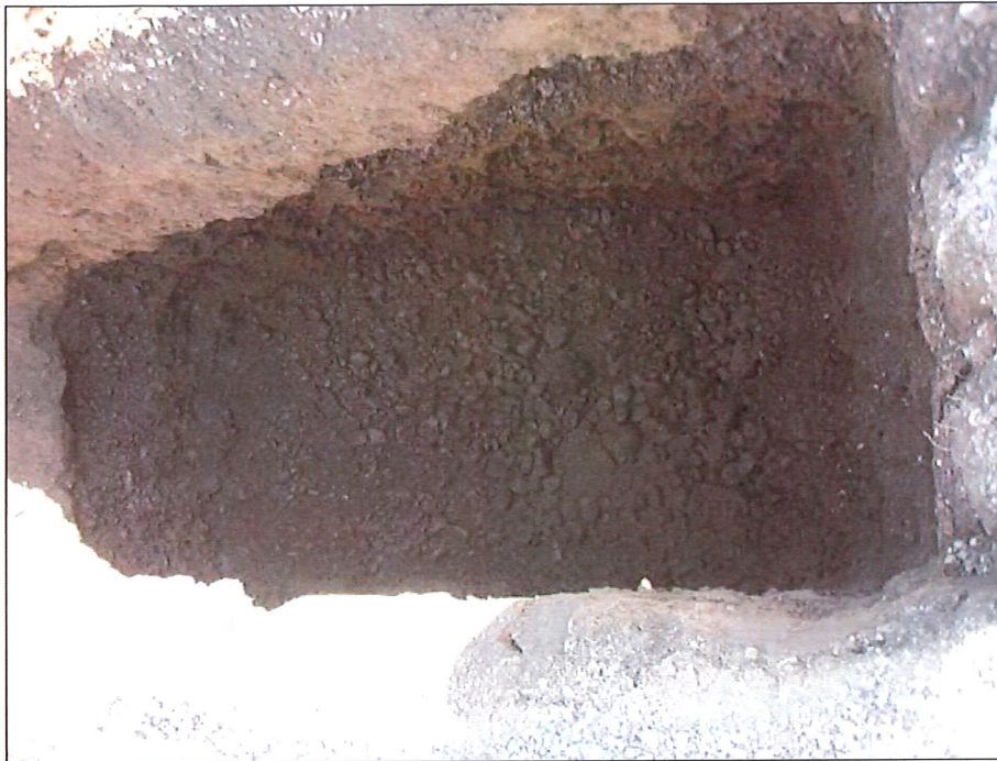
Photo 1: Test Pit TP1- Silty Gravel to Gravel Deposit
