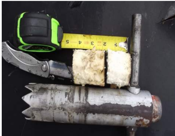
Roof Core Pool Corridor RA - 15
